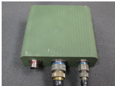
Figure 5 VMU with power and instrumentation cables
